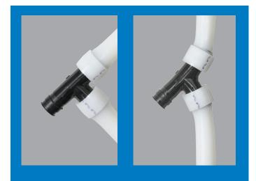
With 3,000 pounds of force and a linear displacement of 13.2", this 2" ProPEX fitting has not been compromised. It can also be noted that the PEX pipe and ProPEX ring have not failed or backed off the fitting.
