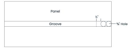
Figure 24: Drill two holes to create a rectangular slot in the subfloor.
