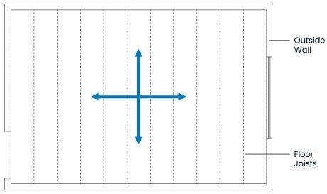
Figure 16: For a wood-finished floor covering, install Quik Trak panels perpendicular to the direction of the finished-wood floor boards.
