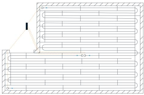
Figure 13: Manifold location in the joist cavity
