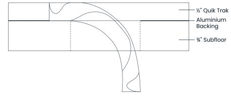
Figure 25: Trim aluminum backing to allow bend support to be flush with the top of the panels.
