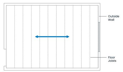
Figure 14: For tile, parquet, and linoleum finished floors, install Quik Trak panels perpendicular to the floor joists. This will add strength to the floor and help prevent deflection of the floor.
