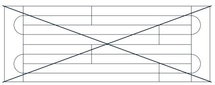
Figure 22: Incorrect panel placement
