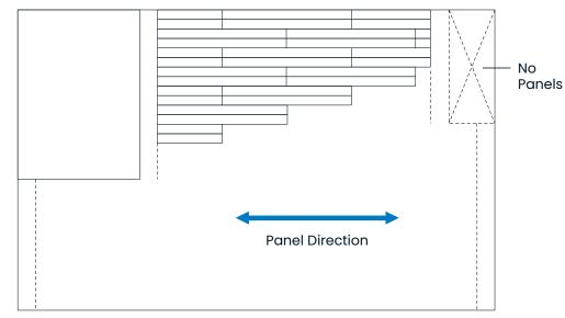
Figure 18: Stagger panels so seams do not line up.
