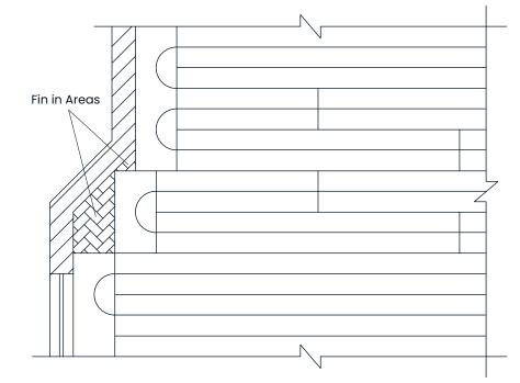
Figure 23: When installing the panels in a room with an alcove or bay area, remember to allow enough room for the return panels. Fill any areas not covered with panels with ½" plywood.
