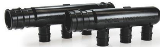
The new multiport tees feature 1 1/4" inlets and three 3/4" outlets and are designed for commercial installations where supply lines are required to be upsized due to pressure or code requirements.
