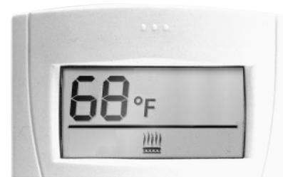
Figure 1: Thermostat display indicating call heat.
