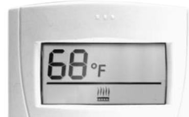
Figure 1: Thermostat display indicating call heat.
