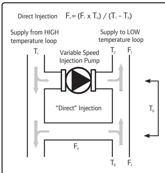
**Figure I-2: Direct Injection Mixing ( $F_V$  Formula)**
