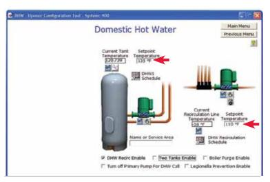
Figure 2.8-6: Single DHW Tank with Recirculation
