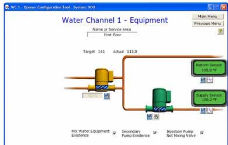
Figure 2.9-5: Injection Pump Mixing Screen
