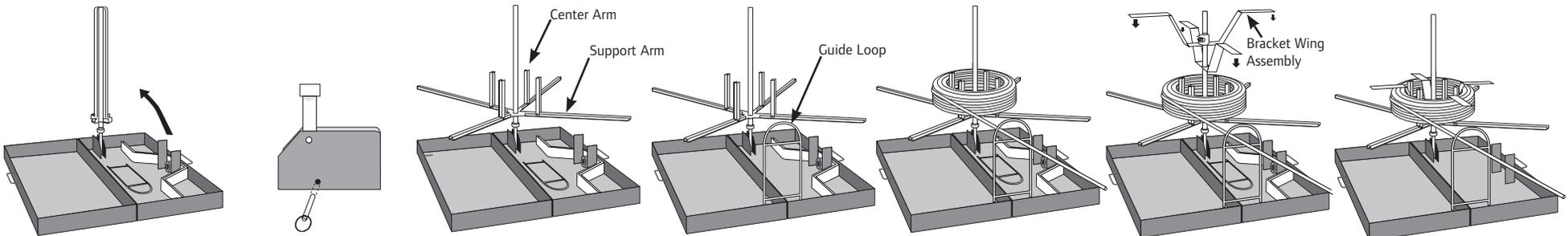
1. Lay the case open and raise the main tower shaft assembly.
