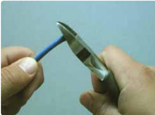
**Figure A.5-1: Cutting the Cable Wiring**
