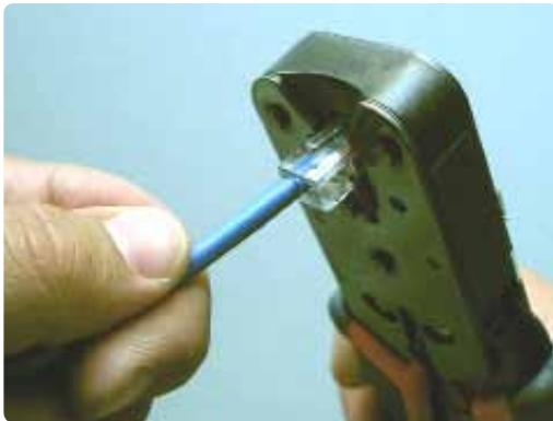
**Figure A.5-10: Crimping the Wire Assembly**
