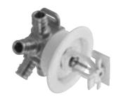
The Concealed Sprinkler Assembly comes with the sprinkler threaded onto Uponor's stainless steel multi-port fitting with ProPEX outlets. All assemblies come complete with a plastic protective cap and cup. Sprinkler assemblies are NSF- and UL-approved for combined plumbing and sprinkler systems.
