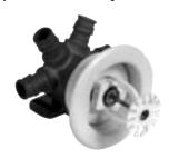
The Recessed Pendent Sprinkler Assembly comes with the sprinkler threaded onto the stainless steel multi-port fitting with ProPEX outlets. All assemblies come complete with a protective plastic cap and escutcheon. Sprinkler assemblies are NSF- and UL-approved for combined plumbing and sprinkler systems.
