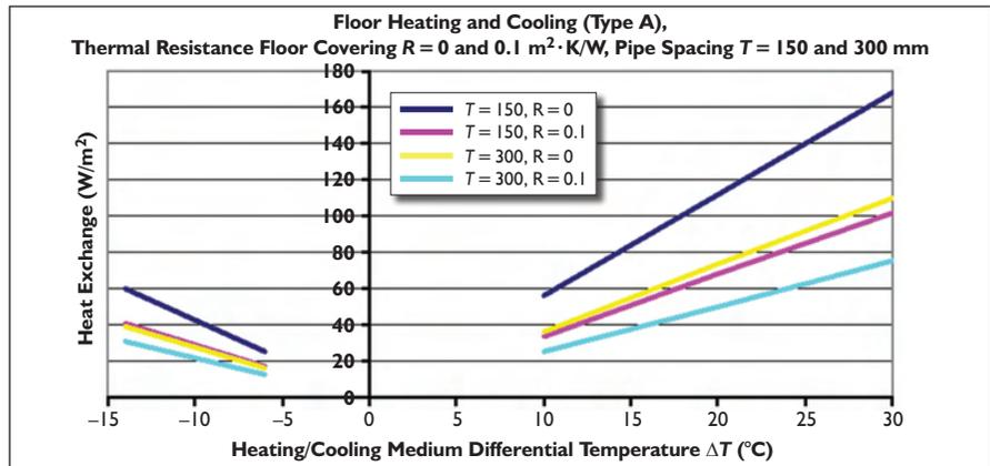
Figure 2: Heat exchange expressed as the function of  $\Delta T$  between water and room, type of floor covering (R), and pipe spacing (T). Carpet:  $R=0.1 \text{ m}^2 \cdot \text{K/W}$  and no covering  $R=0$ .
