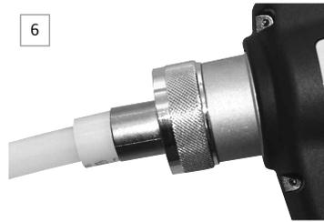
6. Repeat the expansion process until the tubing and ring are snug against the shoulder on the expander head. See **Table 1** on page 3 for the recommended number of expansions for each tubing size.
