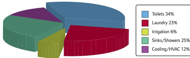
Reclaimed water systems eliminate approximately **60%** of potable demand (for toilets, laundry and irrigation).\*
