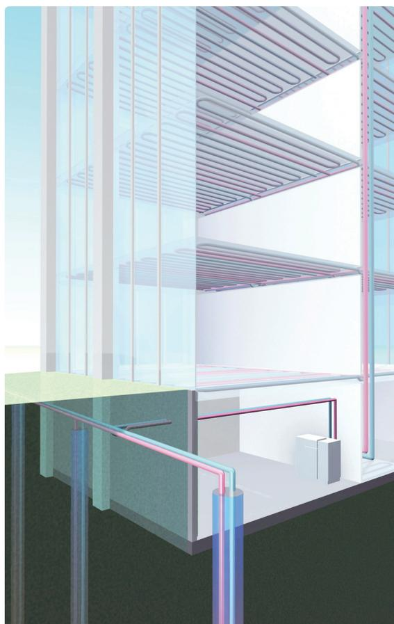
Comfort is ensured by optimal temperatures provided by a silent system that does not circulate air: no dust, no draughts – ensuring a healthy indoor environment. The invisible system also gives freedom of space and flexible indoor design.
