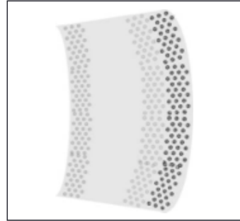
Figure 1-2: PEX-b (Silane) 65-70% crosslinked
