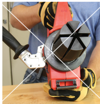
Figure 2-12: Incorrect expansion head "flowering"
