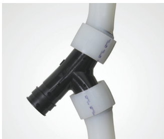
Figure 1-7: At approximately 2,900 lbs. of pull force
