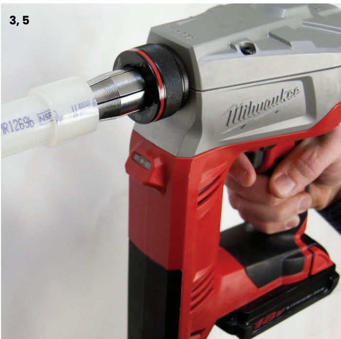
Figure 2-9: Expansion with Milwaukee M18 ProPEX Expansion Tool
