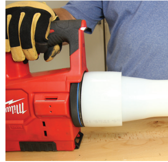
Figure 2-18: Expand to shoulder
