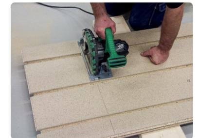
The panels are easily cut with a circular saw.
