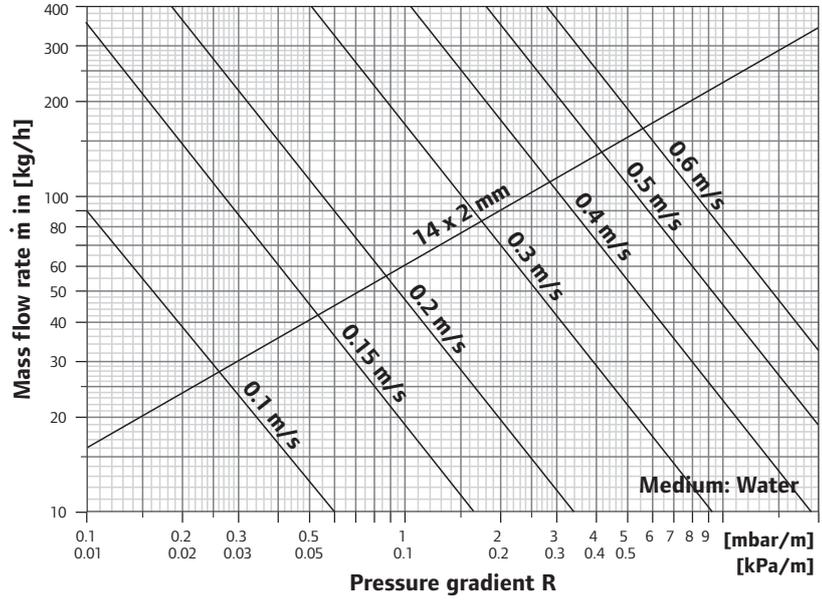
The pressure losses in the Uponor multi-layer composite pipes can be determined with the aid of the diagram
